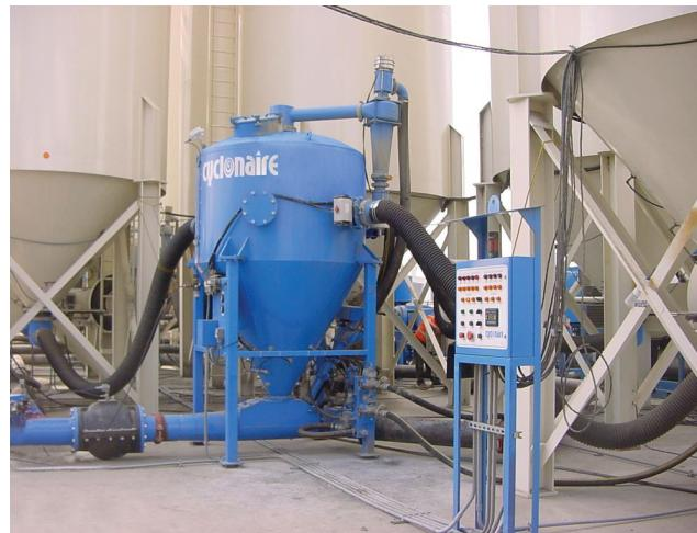
A PLC control panel shown in the foreground provided automatic cycling and condition monitoring for operating the HC systems.
