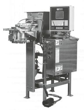
bagger for filling open-mouth bags, boxes and drums with dry powdered, pelleted or granular materials.
