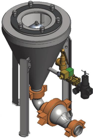
**Simple Dust Reclaim** – The CycloLok is a gravity loaded, bottom discharged low-volume, dense phase conveyor with only one moving part. It is best suited for highly abrasive and friable materials in especially harsh environments, such as high temperature dust reclaim.
