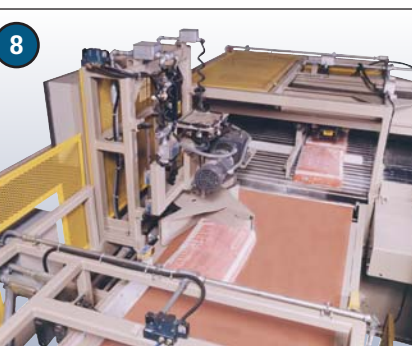
PATENTED BAG TURNWHEEL LAYER FORMING CONVEYOR/LAYER PUSHER Pop-up bag stops separate bags to maintain shape. Retractable pusher plate moves half layers onto stripper plate, then swings up on the return cycle, allowing the next half layer to be forming while the first is being placed. Available with optional indexing belt.
