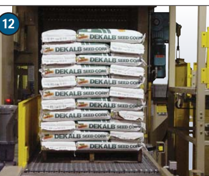
FILLED PALLET CONVEYOR Gravity conveyor with holding space for three filled pallets is standard. Powered steel mesh belt and roller conveyors are available for staging pallets or for movement into an automatic stretch wrapper.
