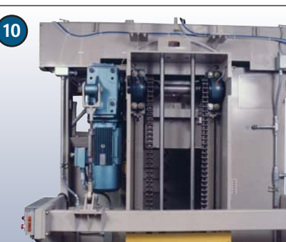
MAINFRAME/HOIST Sew-Eurodrive motor provides smooth operation of the hoist. Standard 4000-pound load uses 12.5 HP motor and #100H chain. Heavier loads can be accommodated. Counterweights are used to offset some of the load and provide constant chain tension.
